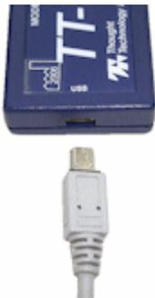
Insert the small connector of the USB cable into the USB port on the TT-USB interface device.
