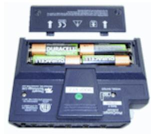
**Attention:** *The internal workings of the ProComp5 Infiniti encoder are not intended to be opened for repair except by qualified service personnel. The tamper-evident seal under the batteries in the battery compartment should not be removed or broken.*
