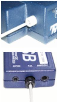
Insert one end of the fiber optic cable carefully into the fiber optic port on the encoder. Tighten the nut gently so that the cable won't slip out.
