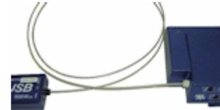
**Note:** The fiber optic connectors may break if they are hit directly, for instance, if the encoder falls onto the floor. To prevent damage, it is recommended to use the encoder belt clip to fasten it to the client or to a chair.
