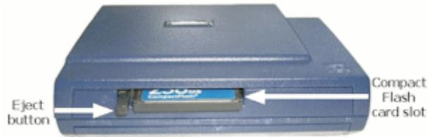
To remove the insert, push the button next to the slot once to eject it. The card can then be inserted, as shown. To protect from incorrect insertion the card can be inserted into the device only one way. When inserted properly it is flush with the device rear.
